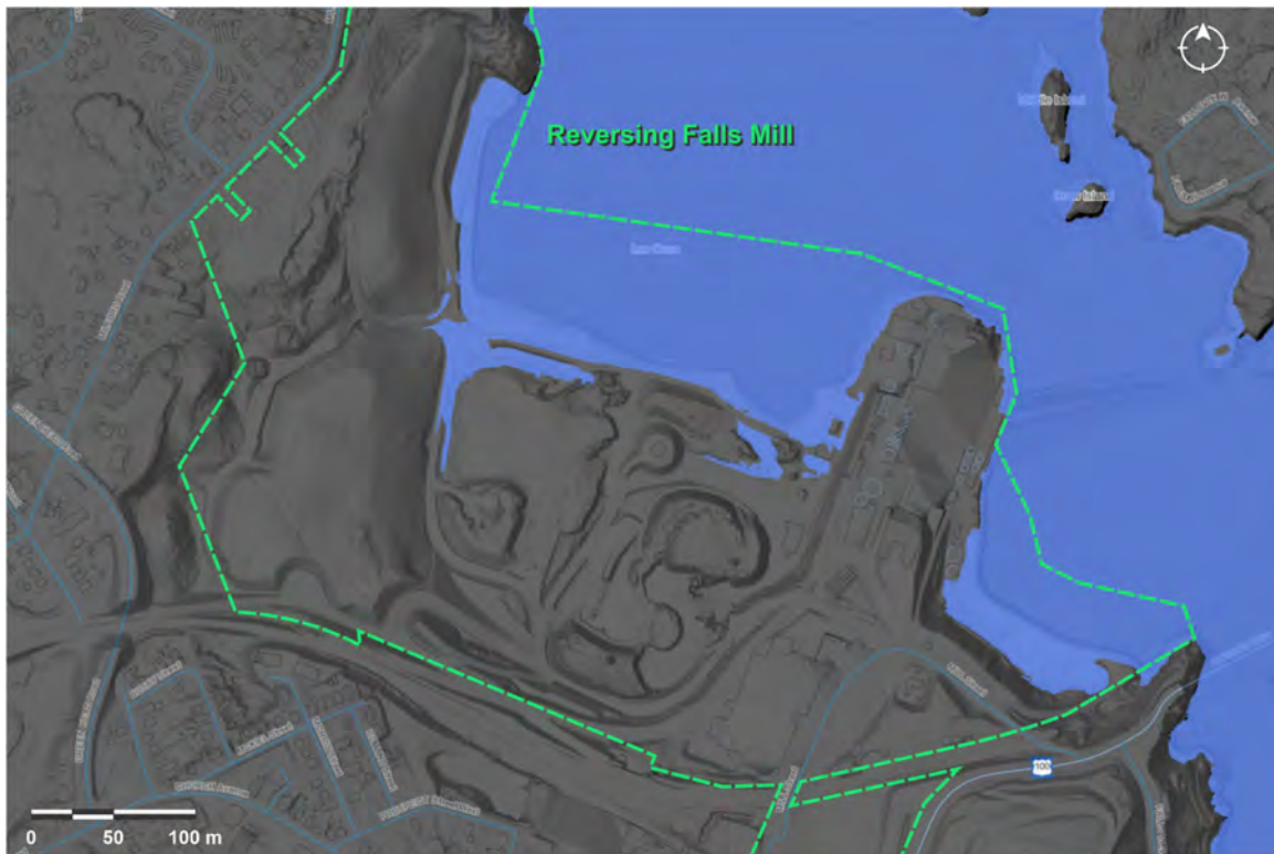
Figure 109. Land in vicinity of the Reversing Falls Mill in Saint John, New Brunswick that currently floods during a 1 in 20 year flood event.
