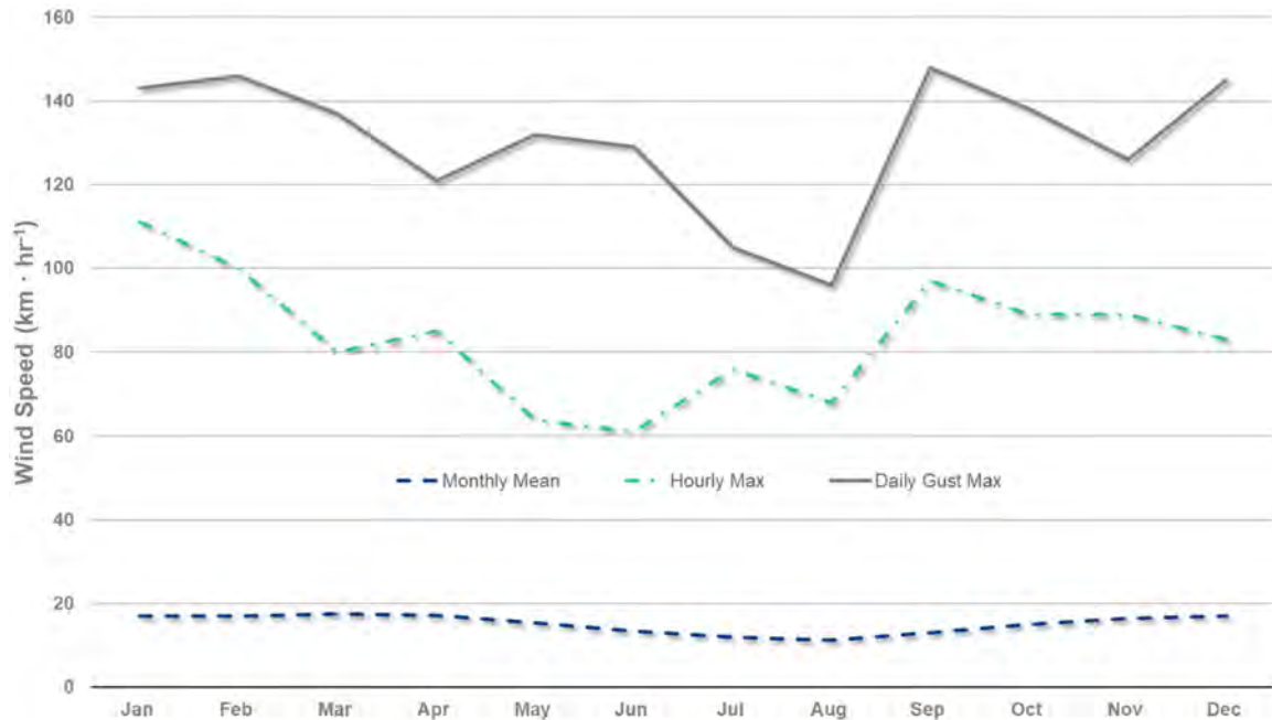
Figure 39. Compilation of wind speeds measured for the 30 year period between 1981 and 2010 at Saint John Station A ( i.e. , Saint John airport).
