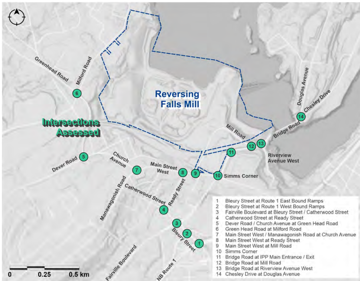
Figure 97. Intersections where traffic volumes were collected by Englobe staff in October 2022 to provide AM and PM peak hour turning movement counts near the Reversing Falls Mill in Saint John, New Brunswick.
