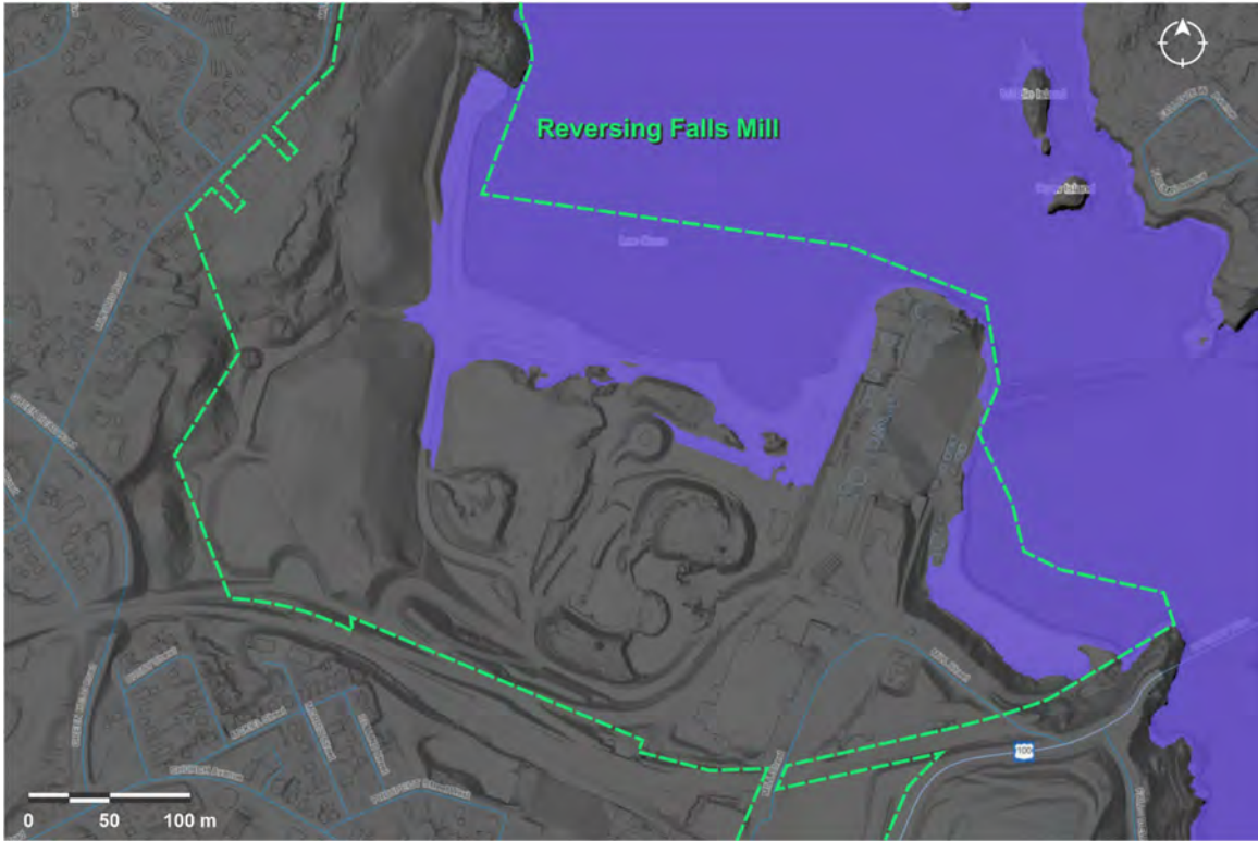
Figure 110. Land in vicinity of the Reversing Falls Mill in Saint John, New Brunswick that currently floods during a 1 in 100 year flood event.
